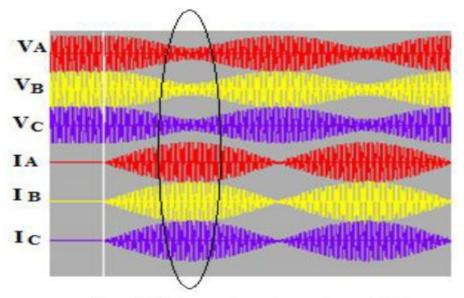
Figure 14. Voltage and current curve forms at OOS
