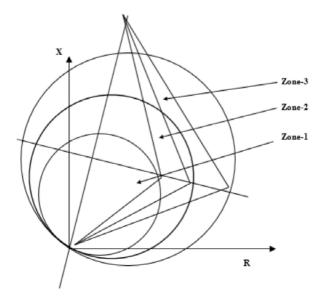
Figure 12. Three stepped distance protection
