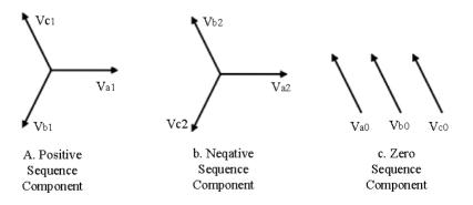
Figure 2. Analyze the sequence component in the power system
