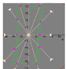
Figure 19. Test relay OOS function boundary graph for the outer zone
