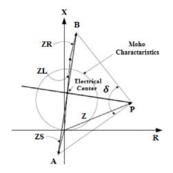
Figure 9. Intelligent relay characteristics Impedance trajectories at OOS
