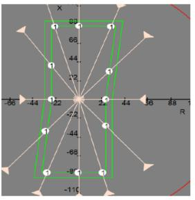
Figure 18. Test relay OOS function boundary graph for the inner zone
