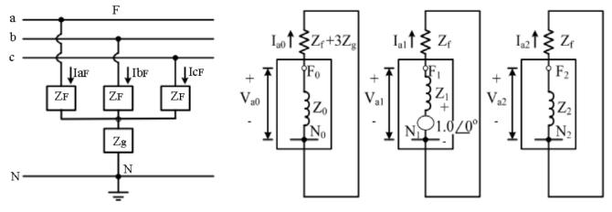
Figure 3. General simulation of a three-phase fault
