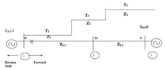
Figure 11. Single line diagram showing three protection zones
