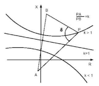
Figure 10. Impedance Trajectories at relay point during power swing
