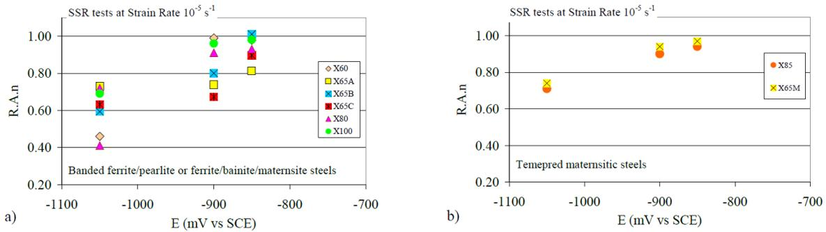
**Figure 5.** Normalised reduction of area after SSR tests in synthetic sea water under cathodic protection at  $10^{-5} \text{ s}^{-1}$  strain rate vs applied potential
