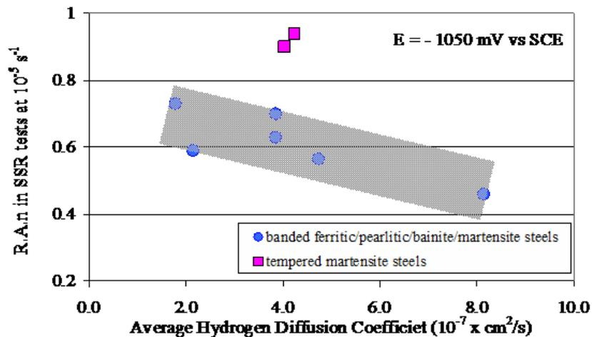
**Figure 6.** Normalized reduction of area in SSR tests in sea water under cathodic protection at strain rate  $10^{-5} \text{ s}^{-1}$  as a function of the average hydrogen diffusion coefficient
