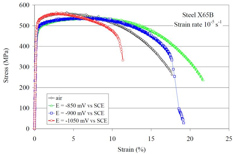
Figure 3. Stress vs strain curves obtained in the SSR tests on the specimens of X65B steel in artificial sea water under cathodic protection at strain rate  $10^{-5} \text{ s}^{-1}$  and different applied potential.
