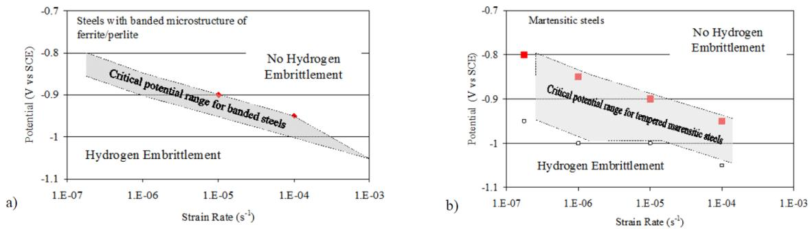
**Figure 4.** Effect of strain rate on critical potentials for hydrogen embrittlement
