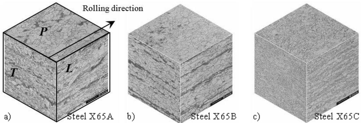
**Figure 1.** Microstructure of the X65 steels
