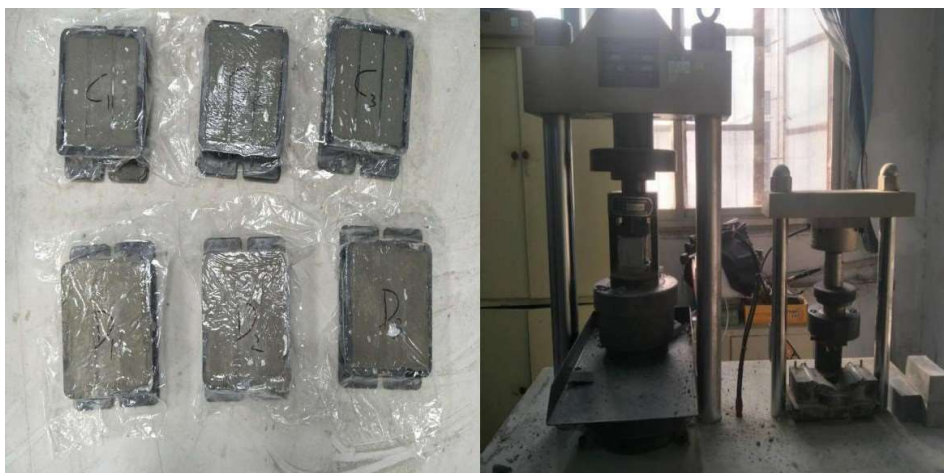
Figure 4. Grouting material test block.
