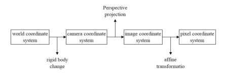
Figure 5 Camera imaging coordinate system conversion
