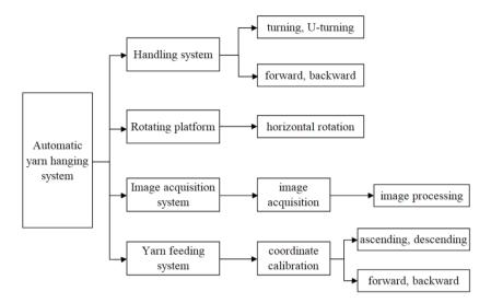
Figure 1 Block diagram of automatic yarn hanging system
