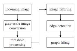
Figure 2 Image processing flowchart
