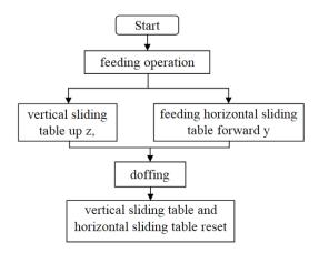
Figure 6 Flow chart of yarn hanging on sliding table
