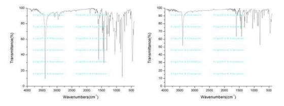
**Figure 2.** The left side shows the infrared spectra of the prepared 2,7-dibromocarbazole; the right is the infrared spectrum of the standard 2,7-dibromocarbazole
