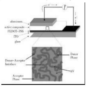
Figure 1. Polymer solar cell structure
