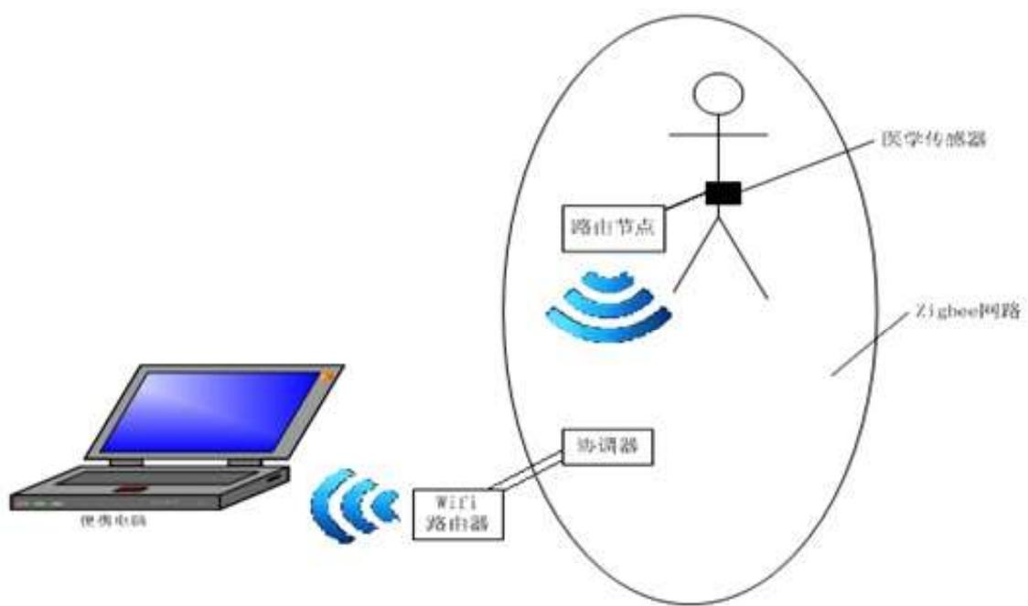
Figure 2. Health monitoring system for wireless networks
