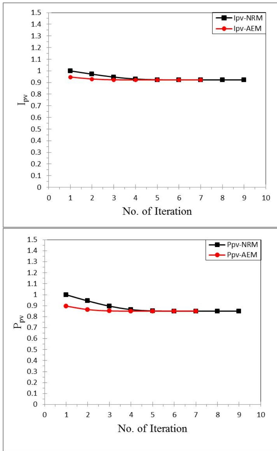
**Figure 3.** Number of iterations vers the solar cell parameters  $I_{pv}$ ,  $P_{pv}$  and  $V_{pv}$  using NRM and AEM.
