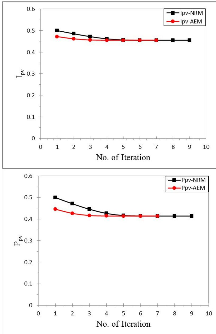
**Figure 5.** Number of iterations vers the solar cell parameters  $I_{pv}$ ,  $P_{pv}$  and  $V_{pv}$  using NRM and AEM.
