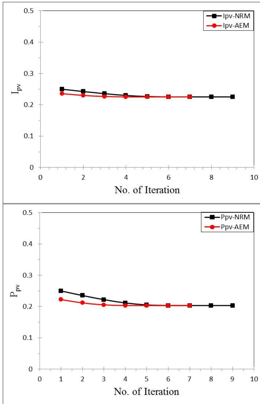
**Figure 6.** Number of iterations vers the solar cell parameters  $I_{pv}$ ,  $P_{pv}$  and  $V_{pv}$  using NRM and AEM.
