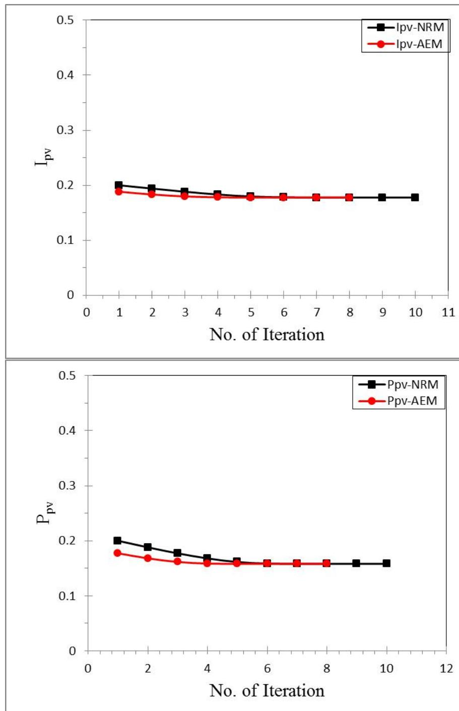
**Figure 7.** Number of iterations vers the solar cell parameters  $I_{pv}$ ,  $P_{pv}$  and  $V_{pv}$  using NRM and AEM.
