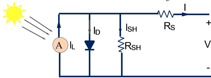
**Figure 1.** PV-cell equivalent-circuit models: single-diode model.
