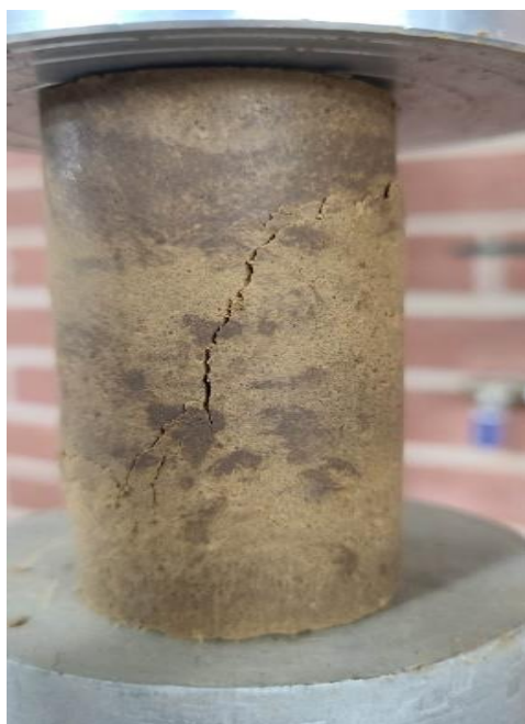
Figure 2. UCS failure mode of a 10% water content soil mixture.
