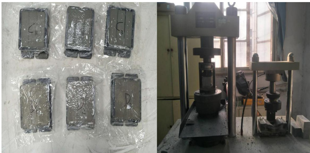
Figure 4. Grouting material test block.
