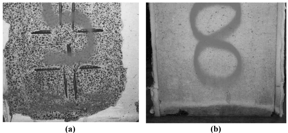
Figure 7. Efficiency of polypropylene fibers. (a) Concrete without fibers; (b) concrete with polypropylene fibers [27].
