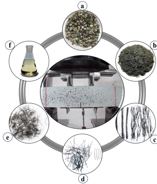
Figure 2. Raw materials of FRS: (a) Fine Sand (FS); (b) Cement (C); (c) Forta Fiber (FF); (d) 3D hooked-end Manufactured Steel Fiber (MSF); (e) Recycled Steel Fiber (RSF); (f) Super Plasticizer (SP).
