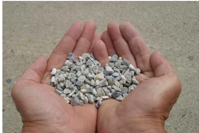
Figure 30. Dolomit Chippings 4/8 mm LSK as bedding material [25].
