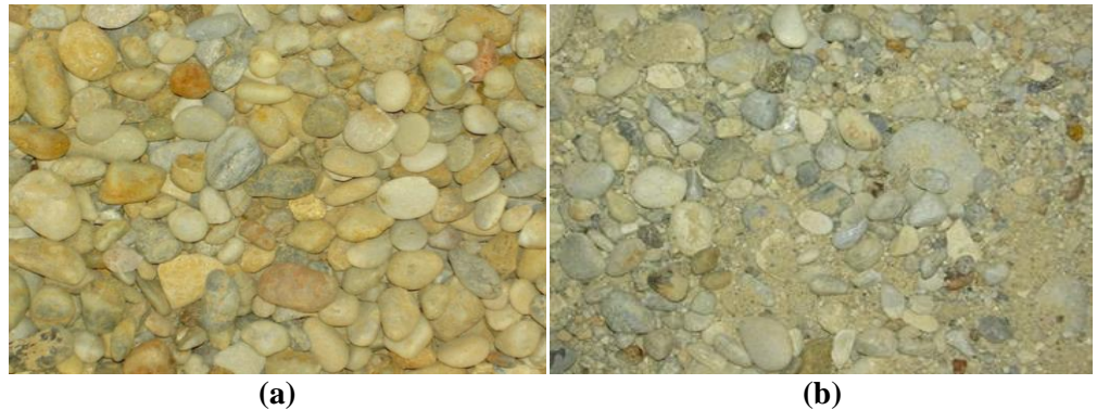
Figure 11. (a) Self-graded gravel (GE); (b) coarse-grained, non-cohesive soils (Gravel or sand) (GW, GI, SE, SW, SI) [8].
