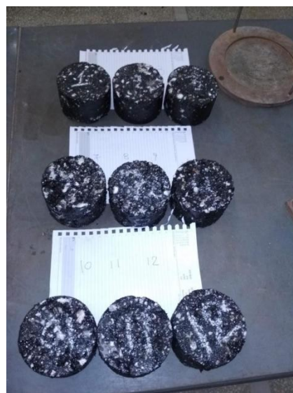
Figure 3. Asphalt mix specimens with LDPE waste.
