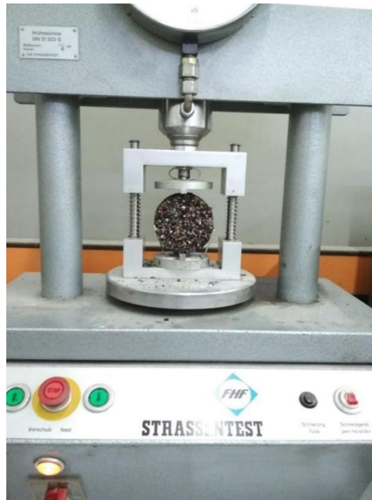
Figure 2. Indirect tensile test.
