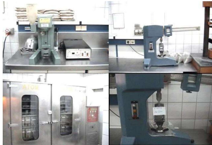
Figure 2. Equipment for preparation and testing of mortar composite, left to right, the automatic-minute-controlled mixer, the bending moment testing machine, curing cabinet whose relative humidity and water temperature is controlled by computer, bending moment testing of mortar composite containing MP.
