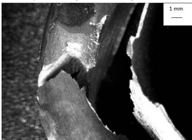
Figure 8. Failed specimen showing delay failure and splitting due to crack propagation
