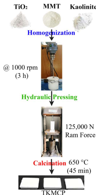
Figure 1. Major steps employed in TKMCP blocks fabrication.
